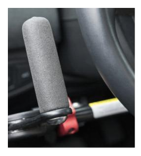
Modifications include hand controls for the gas and brakes.
