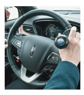
An adaptive spinner knob can help with steering (above and below).
